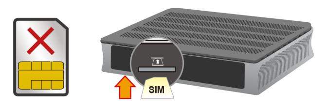
WARNING: Please power off the device before inserting or removing the SIM
