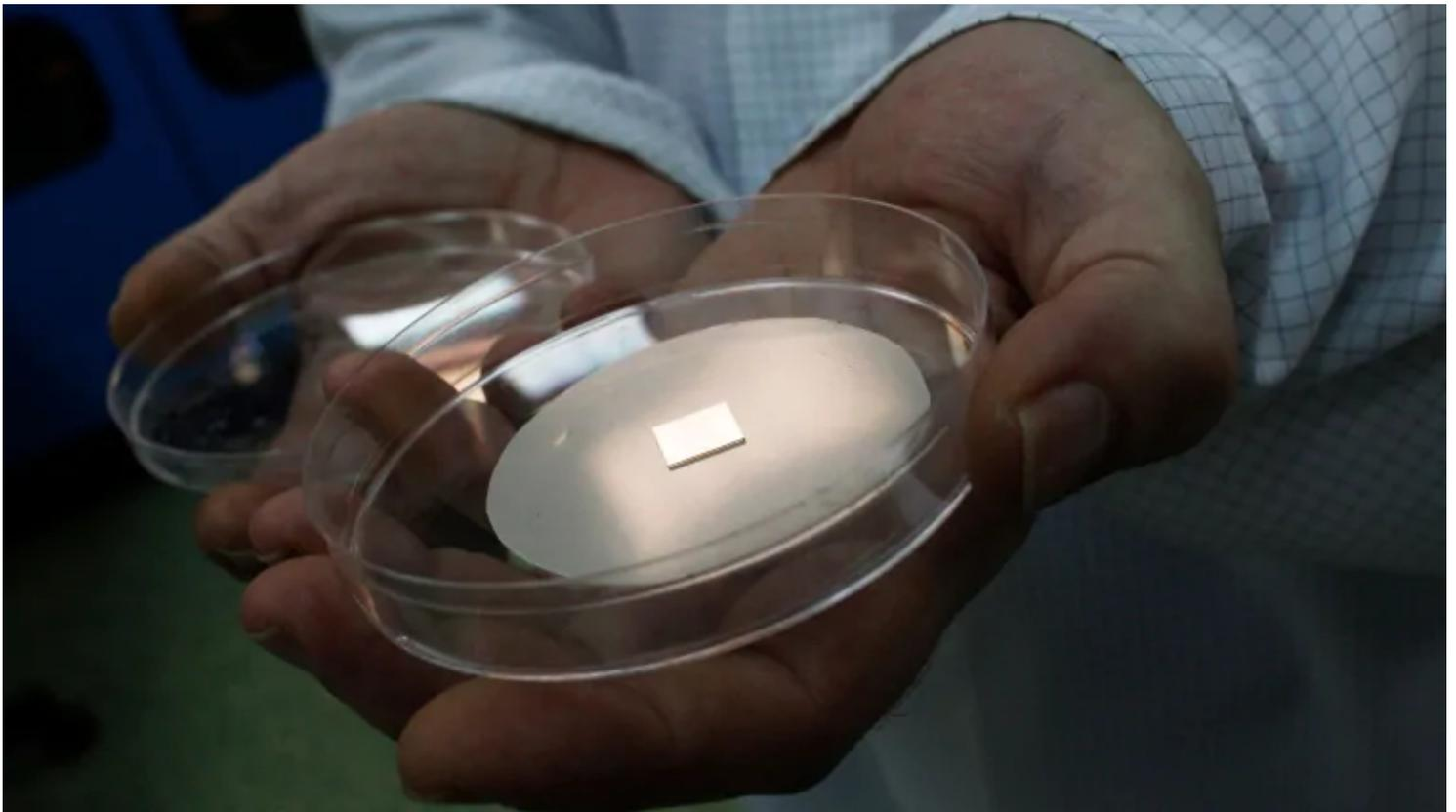
Senior technologist Dariusz Czolak holds a piece of silicon carbide disk covered with a layer of graphene, a material that can conduct electricity with very little resistance, in 2012. (REUTERS)
