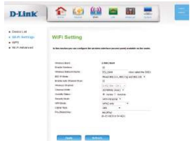
**Channel Width:** A higher channel width allows for faster data transmission, at the possible expense of wireless coverage and compatibility with older wireless clients. Select the optimum channel width for your wireless network from the drop-down menu.
