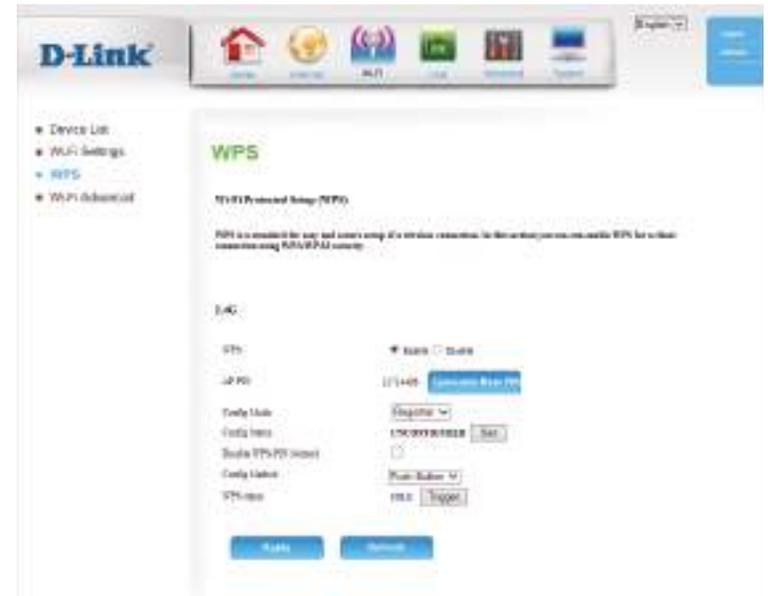
**Config Method:** This lets you choose whether to use the **Push Button** connection method (PBC) or **PIN** method to connect to a wireless client when the **Trigger** button is clicked. If you choose the **PIN** method, you will need to enter an 8-digit PIN number that the wireless client needs to use to connect to your router.
