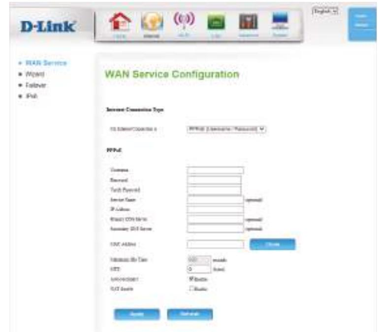
**Auto-reconnect:** The device will automatically reconnect to your PPPoE connection automatically.
